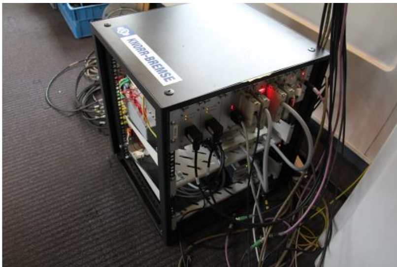
Figure 4: Additional electronics installed in parallel with the original brake control hardware were used to implement the new functions and algorithms. Source: Knorr-Bremse Systeme für Schienenfahrzeuge GmbH
