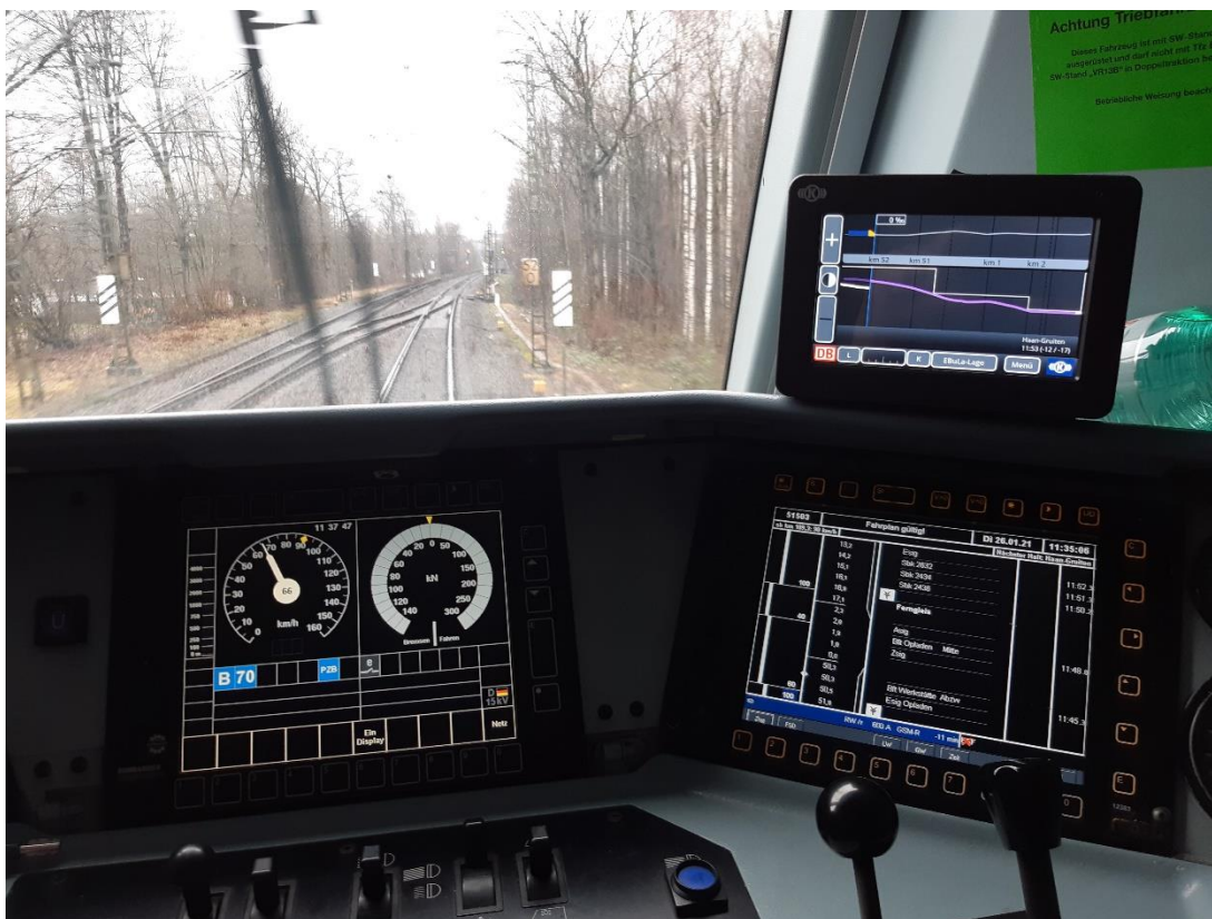
Figure 1: Real-world data from DB Cargo's LEADER DAS can be used to generate robust forecasts of the energy savings which interested RUs can expect to achieve.
