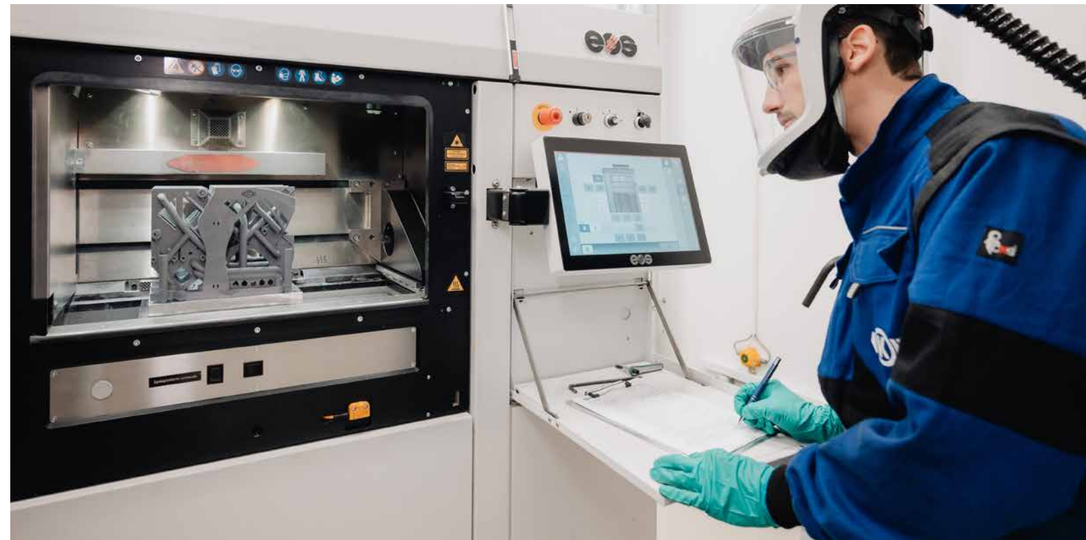
ONCE THE PRINTING PROCESS is complete, the product is removed and cleaned.
