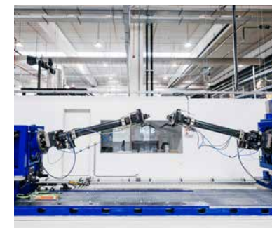
IN-HOUSE testing infrastructure for coupling systems at Knorr-Bremse's Budapest facility
