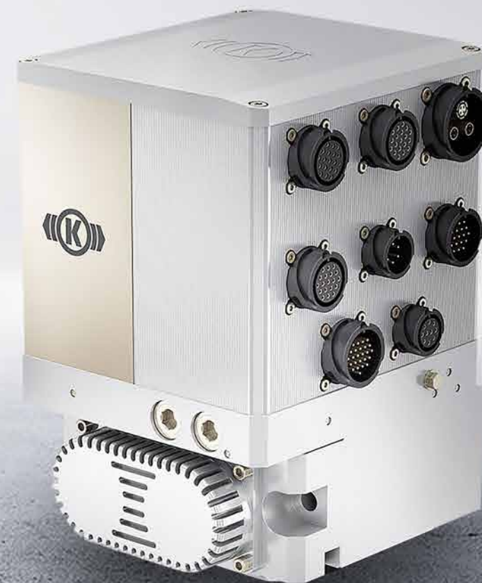
ALSTOM RELIES ON THE LATEST GENERATION OF THE BRAKE CONTROL SYSTEM CubeControl, as well as other Knorr-Bremse technologies. | © Knorr-Bremse
