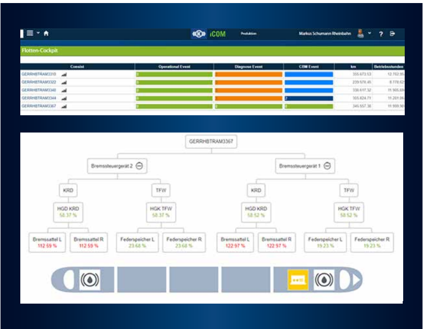
THE FLEET COCKPIT provides an overview of component wear and recent messages
