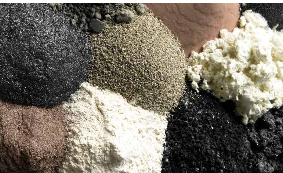
▲ Powders for developing the optimum friction material combination
