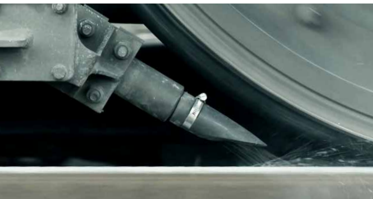
◀ Queensland Rail Australia ▼ Delivering sand to the wheel-rail gap
