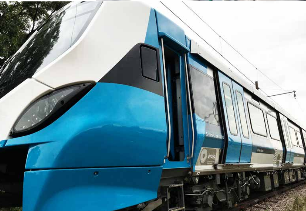
◀ PRASA train with S3 sliding-door system from IFE
