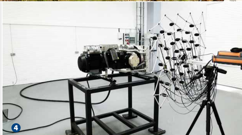
Noise emission analysis of a VV120-T compressor (Figs. 4 and 5). in the acoustic chamber.
