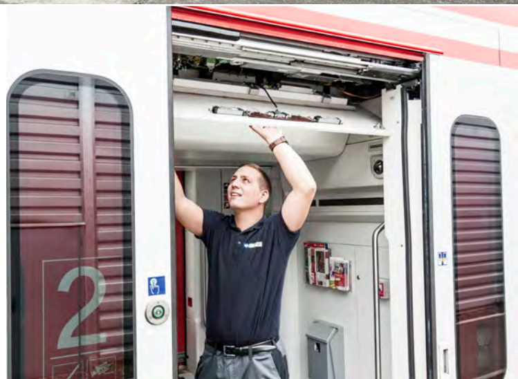
Installation of iCOM into a DB Regio double-decker passenger car.
