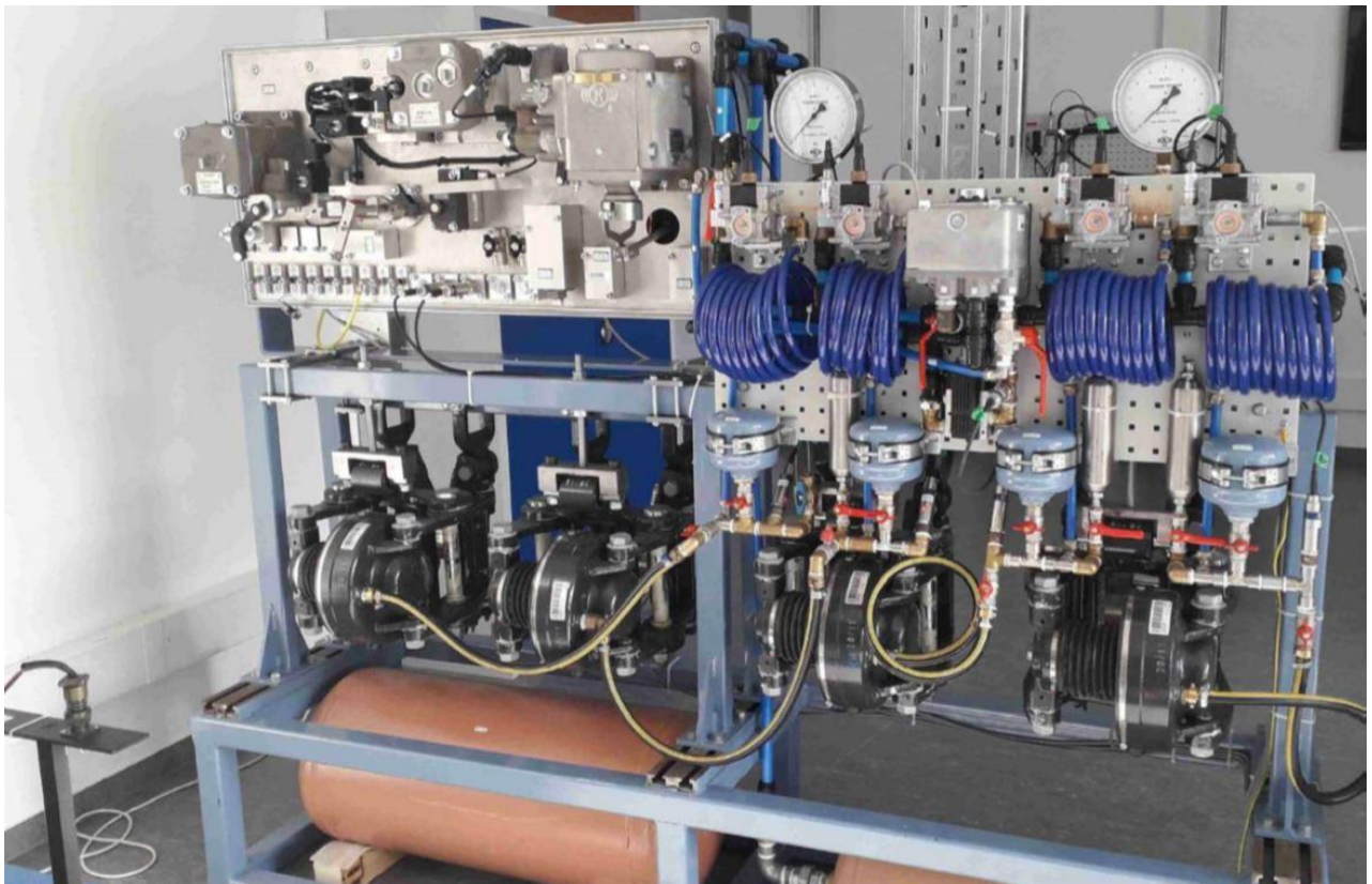
Figure 2: Wheel slide protection system test rig for system optimization
