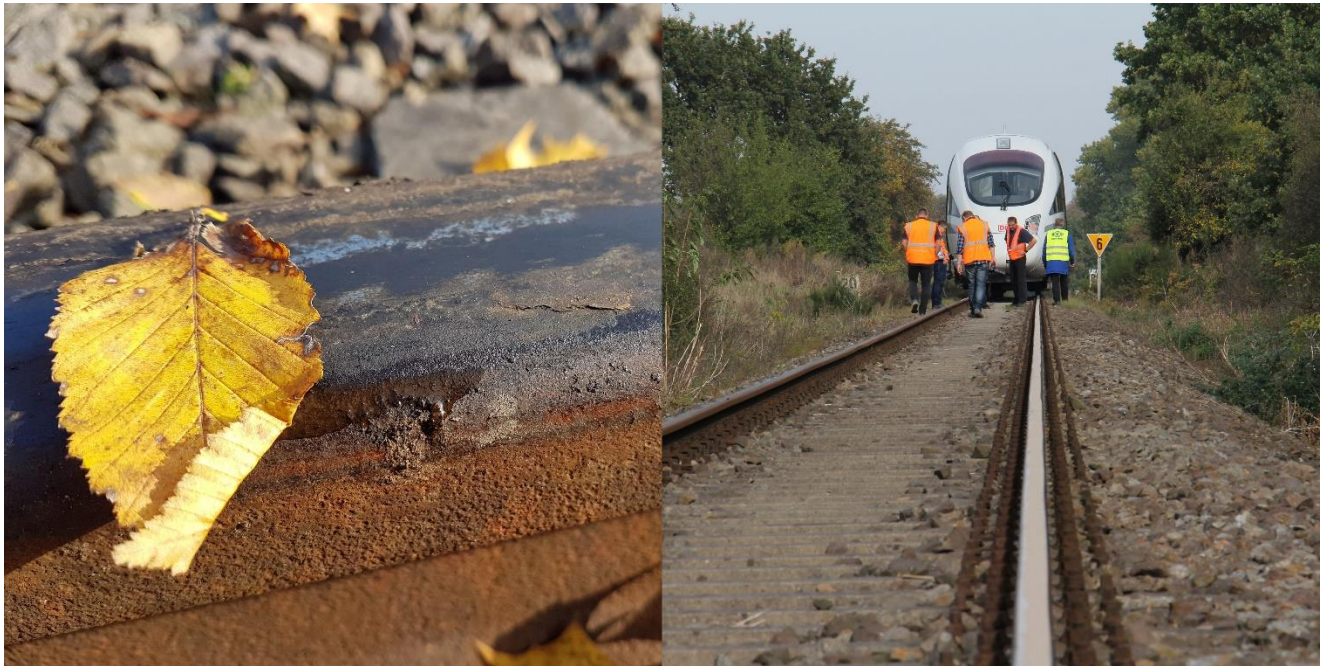
Figure 3: The black leaf layer created by depositing leaves (left) and paper tape (right) provided realistic environmental conditions for the test runs
