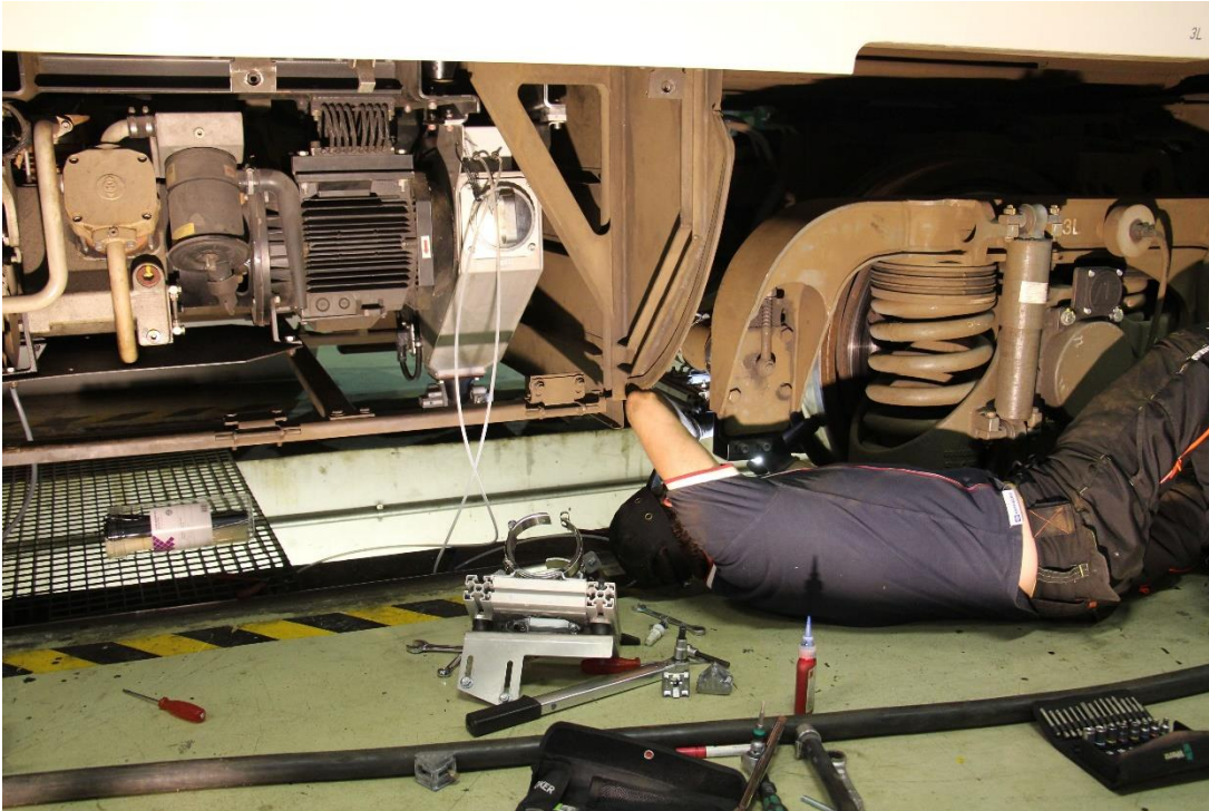
Figure 2: Installation of the dynamically controllable sanding unit in front of the test vehicle's third wheelset
