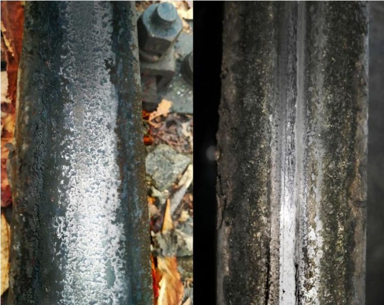
Figure 5: The compacted black leaf layer – in the field (left) and replicated on the wheel-rail adhesion test rig (right).
