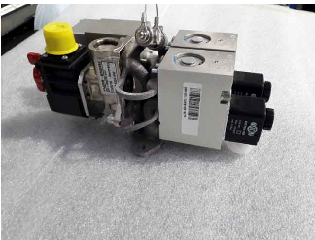
Fig. 4: In order to enable a direct comparison, the 3D-printed function carrier underwent all the standard function test sequences used for conventionally produced panels. The measured values were almost identical to those of conventional panels.
