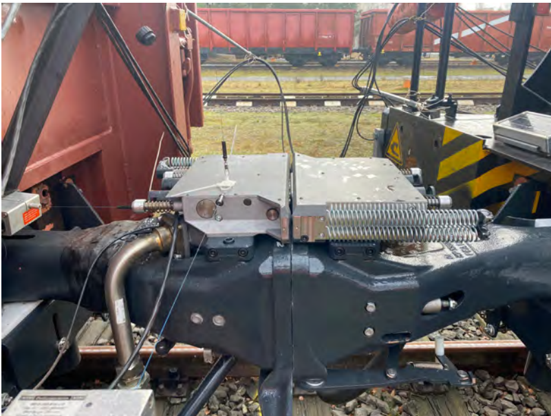
AFTER THE TESTS, TÜV SÜD and the European DAC Delivery Programme approved “FreightLink” (pictured with the prototype electric contact coupler) and gave Knorr-Bremse the go-ahead to test its DAC in a real-world setting.
