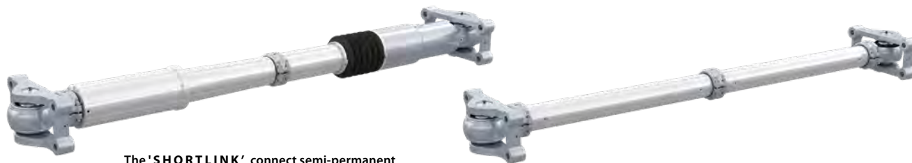
The ' SHORTLINK ' connect semi-permanent couplers the cars within the trainset.
