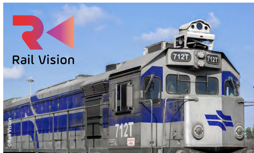
ISRAELI RAILWAY TECH COMPANY RAIL VISION has won an order from Israel Railways to equip passenger and freight trains with high-performance electro-optical sensor systems that alert the locomotive driver in hazardous situations.
