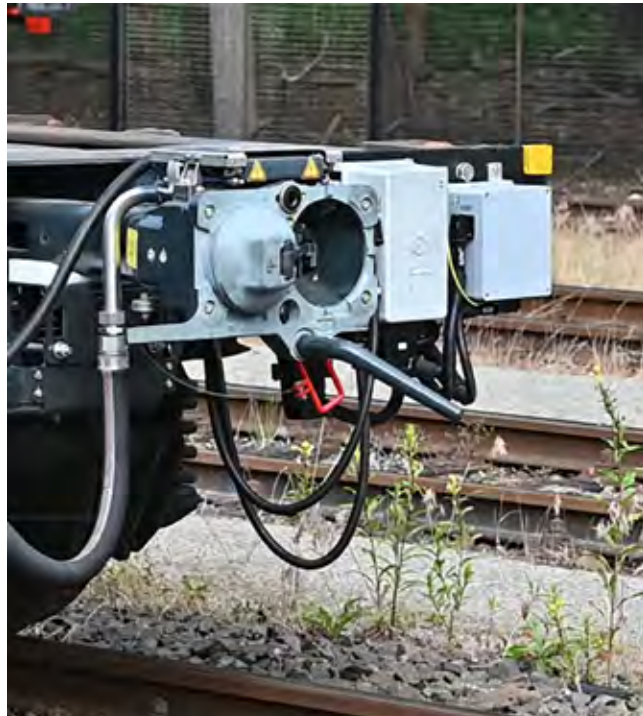
Train Test Laboratory in Berlin-Spandau: A trainset decoupled by remote control for the first time
