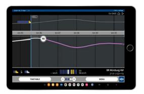
Driver Advisory Systems built into driver's cab runs on a panel PC permanently installed in the driver's cab. Both operators and their personnel benefit from an ergonomically optimized user interface with a clear layout that uses the entire screen to display driving recommendations. This makes interpreting the recommendations as intuitive and stress-free as possible.
