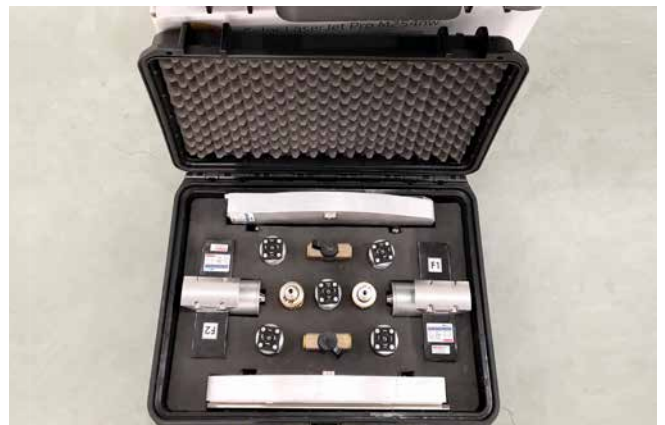
Pressure sensors and force sensors for disk and tread brake
