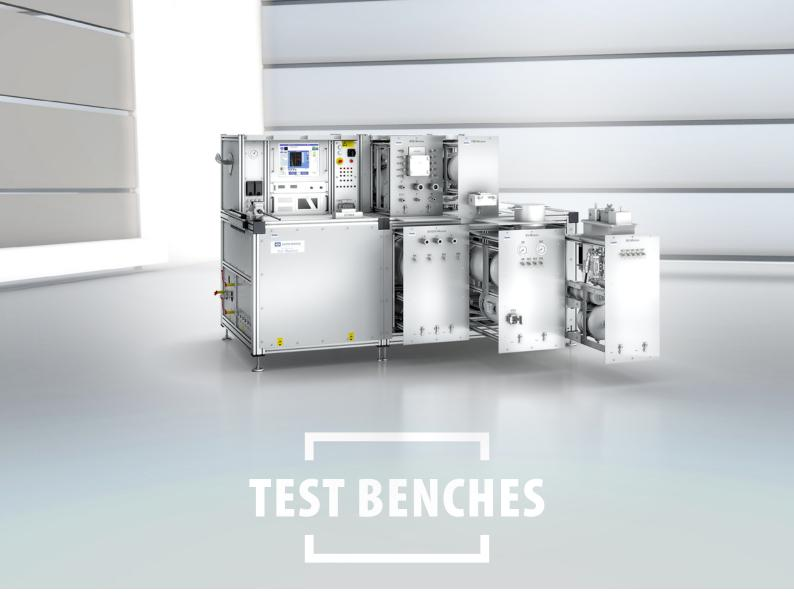
Knorr-Bremse delivers CE-Certified test benches, especially developed for Knorr-Bremse components, to facilitate maintenance and overhaul work and ensure component quality and operational reliability for all types of railroad vehicles. The whole portfolio tests under end of line test instruction (PRF), assuring quality and comparability to original new parts.
