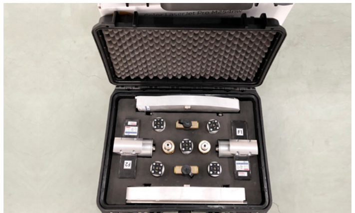
Pressure sensors and force sensors for disk and tread brake
