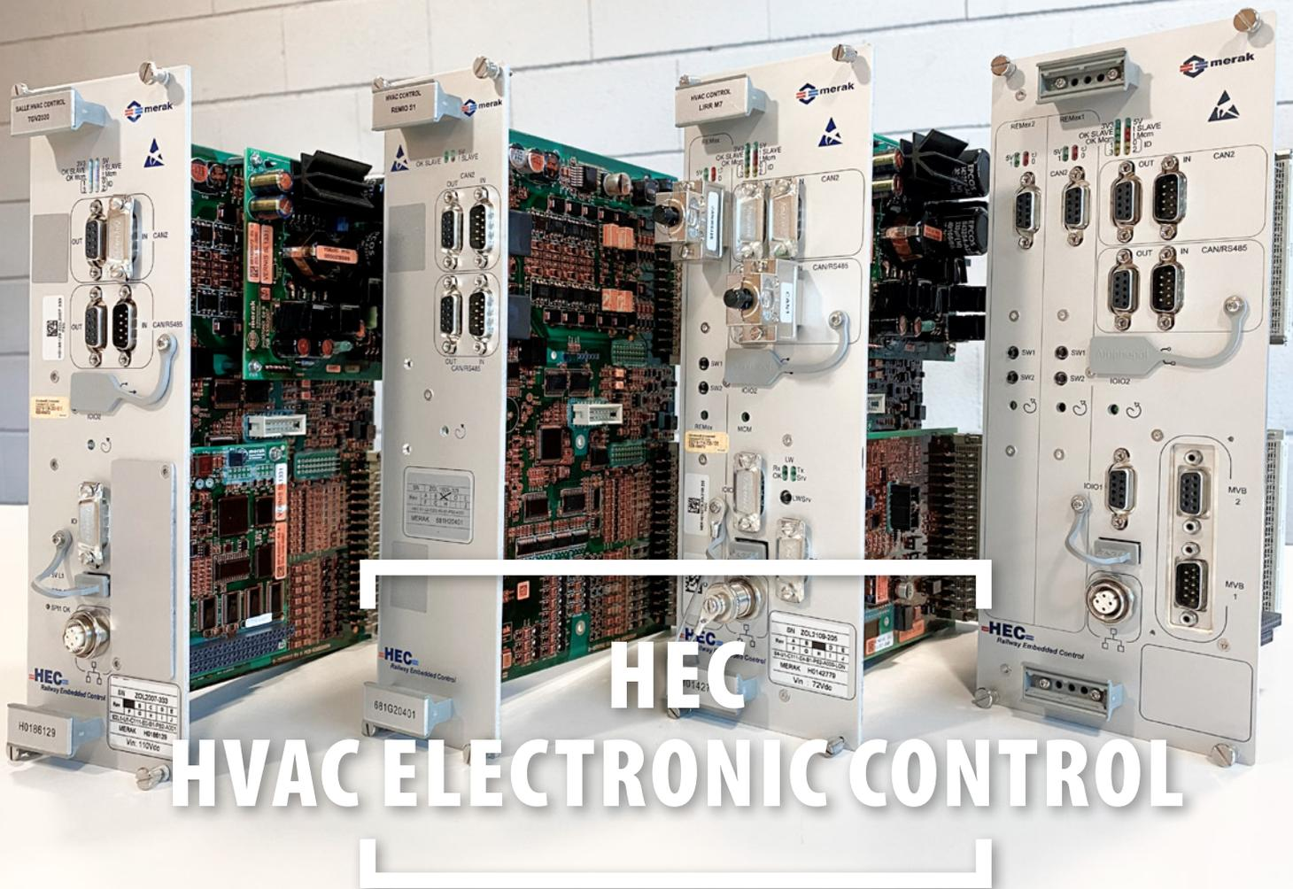
HEC is a state-of-the-art embedded controller designed for railway HVAC applications.
