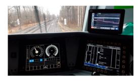
Here, LEADER runs on a panel PC permanently installed in the driver's cab. Both operators and their personnel benefit from an ergonomically optimized user interface with a clear layout that uses the entire screen to display driving recommendations. This makes interpreting the recommendations as intuitive and stress-free as possible.
