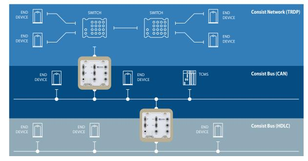
Thanks to the variety of product versions, Selectron Communication Converters are suitable for both retrofits and new fleets. For example, the converters allow the integration of new devices in a legacy technology consist network or they allow legacy devices to communicate over modern networks.
